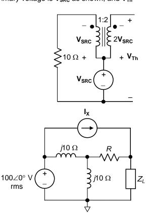
Solution:  $Z_{Th}$  is  $(R + j5) \Omega$ . Hence,  $Z_L$  for maximum power transfer is  $(R - j5) \Omega$ . Version 1:  $R = 5 \Omega$ ,  $Z_{Lmax} = (5 - j5) \Omega$ Version 2:  $R = 6 \Omega$ ,  $Z_{Lmax} = (6 - j5) \Omega$ Version 3:  $R = 7 \Omega$ ,  $Z_{Lmax} = (7 - j5) \Omega$ Version 4:  $R = 8 \Omega$ ,  $Z_{Lmax} = (8 - j5) \Omega$ Version 5:  $R = 9 \Omega$ ,  $Z_{Lmax} = (9 - j5) \Omega$
