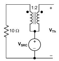
**Solution:** On open circuit, no current flows. The primary voltage is  $V_{SRC}$  as shown, and  $V_{Th} = -V_{SRC}$ .
