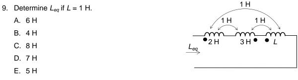
**Solution:** Consider that a voltage V is applied, causing a current I to flow.  $V = j\omega I[(2 - 1 + 1) + (3 - 1 - 1) + (L + 1 - 1)]; L_{eq} = 3 + L.$
