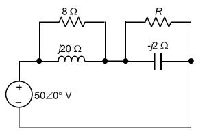
Version 3:  $R = 7 \Omega$ ,  $P_R = \frac{400}{7} = 57.1 \text{ W}$ Version 4:  $R = 8 \Omega$ ,  $P_R = \frac{400}{8} = 50 \text{ W}$ Version 5:  $R = 9 \Omega$ ,  $P_R = \frac{400}{9} = 44.4 \text{ W}$
